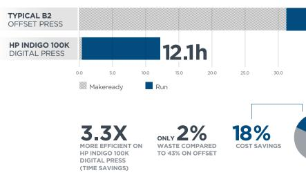
Typical/average B2 offset press in marketplace. Industry Standard/Average Parameters for a two shift operation
